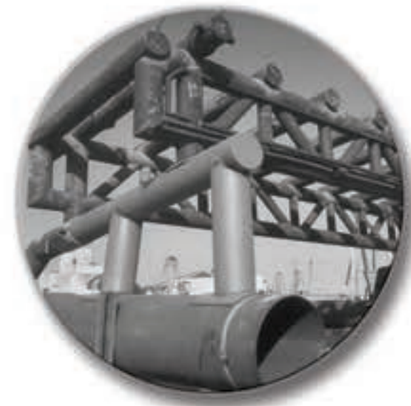
Structural support piping requires proper fit-up of brace members. Weld preparation angles made to stringent AWS specifications enhance structural integrity and reduce grinding and filling labor.
